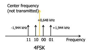
The modulation is constant envelope frequency type, I contrast with TETRA. This imply great advantages in terms of energy consumption: transmitters are very similar to their classic analogical version, expensive linearization is not required, they can work in saturation mode (C class or superior) with energy saving and consumption compatible with solar panels systems. The modulator must have a flat frequency response between 0 and 5 KHz.
