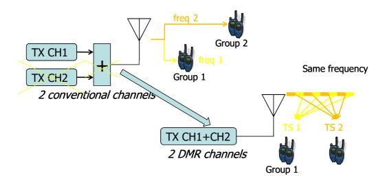
The implemented modulation is 4FSK type (Four-level Shift Keying), optimal for use with PMR communications. Information bits are transmitted by couples, each couple is assigned to a frequency shift
