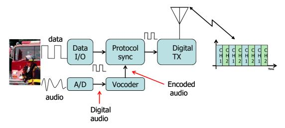
Audio/data channels are managed with two TDMA (Time Division Multiple Access) timeslots sharing the same radio 12.5 KHz wide channel. The two audio/data channel are perfectly separated and independent each from the other, as if they worked in a conventional mode on different frequency (carriers). The transmitter becomes active only during timeslots belonging to their working channel.
