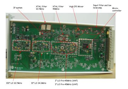
A further input (TX Test input), common for both receivers (main and diversity) is available, for the receiver self-test and for modulator calibration. Through a DSP command, the receiver can switch its input onto test signal generated inside transmission synthesizer module. That signal, amplitude calibrated by Factory, is modulated at receiving frequency and received by DSP. A fundamental test loop is close by this way.
