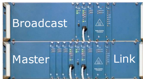
Example of Master station for 4 slaves
