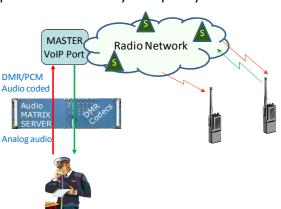
The communication from the mobile terminal is continuously sent to the telephone user (green path in the figure above). The network/repeater sends back the terminal
